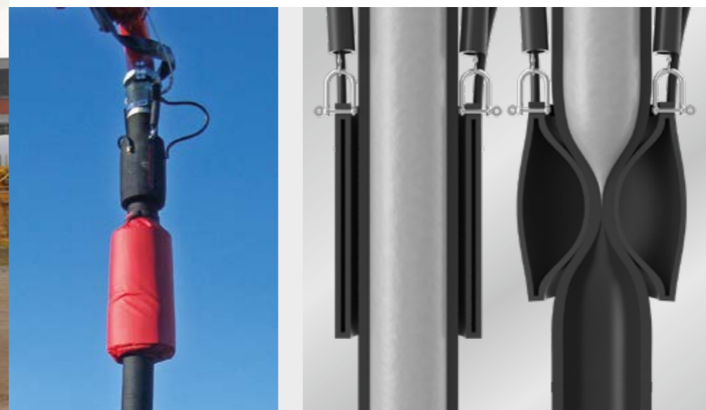
In comparison to the M47, the M46 has less horizontal reach but allows a higher boom tip load. This means that an end hose squeeze valve (EQV) and a divided end hose can be used.
