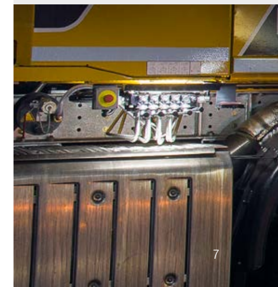
In comparison to the M47, the M46 has less horizontal reach but allows a higher boom tip load. This means that an end hose squeeze valve (EQV) and a divided end hose can be used.
