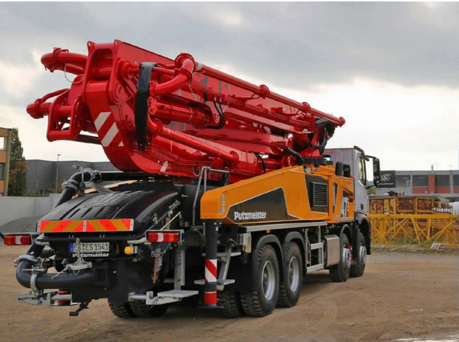
A gross weight of less than 32 t provides a high capacity for payload and functional fluids. This ensures that the machines meet country-specific licensing regulations.
